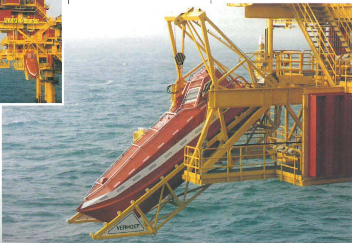
The new NAM L2 gas production platform (insert) is also equipped with an aluminium free-fall lifeboat from Verhoef. (Photo: Hans Janson)
